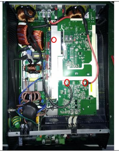
Remove the screws and the signal cables of the MPPT board, and you can take the MPPT board paper off.
