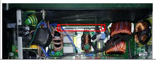
**Note:** When you put the new control board on the main board, please make sure that the connection is correct and tighten. Don't forget to put the screws and cables back.
